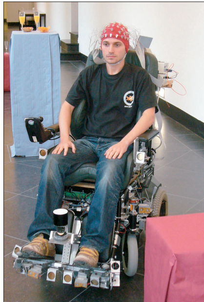
Figure 2. A brain-actuated wheelchair. The subject guides the wheelchair through a maze, using a BCI that recognizes the subject's intent from analysis of noninvasive EEG signals. (photo courtesy of the MAIA project)
